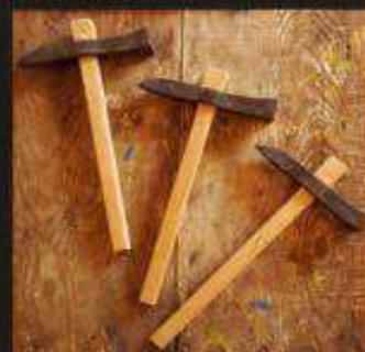
Unique, locally made trullaro hammers, used to work the local limestone and shape chianche .
